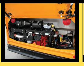
Maintenance shelf allows for quick and easy fluid checks and other routine maintenance.
