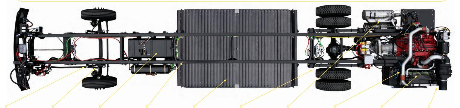
Greaseless front suspension featuring single-stage taper leaf springs (4"x66") with four heavy-duty shock absorbers for outstanding ride quality. Air ride suspensions are available.
