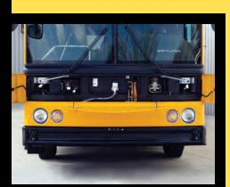
Full-width front access panels open to allow easy access to wiper motors, front heater core and filter, air brake components, chassis wiring connectors and windshield washer fill. Another feature is the recessed optional front crossing control arm, which enhances appearance and reduces the likelihood of damage from minor impact.
