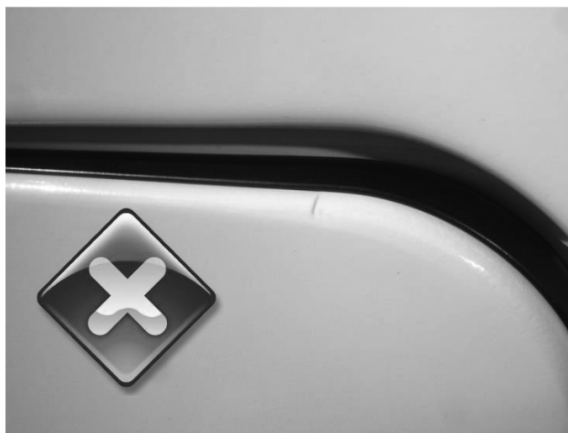
Figure 3: Unacceptable - Door is bent and does not close fully.
