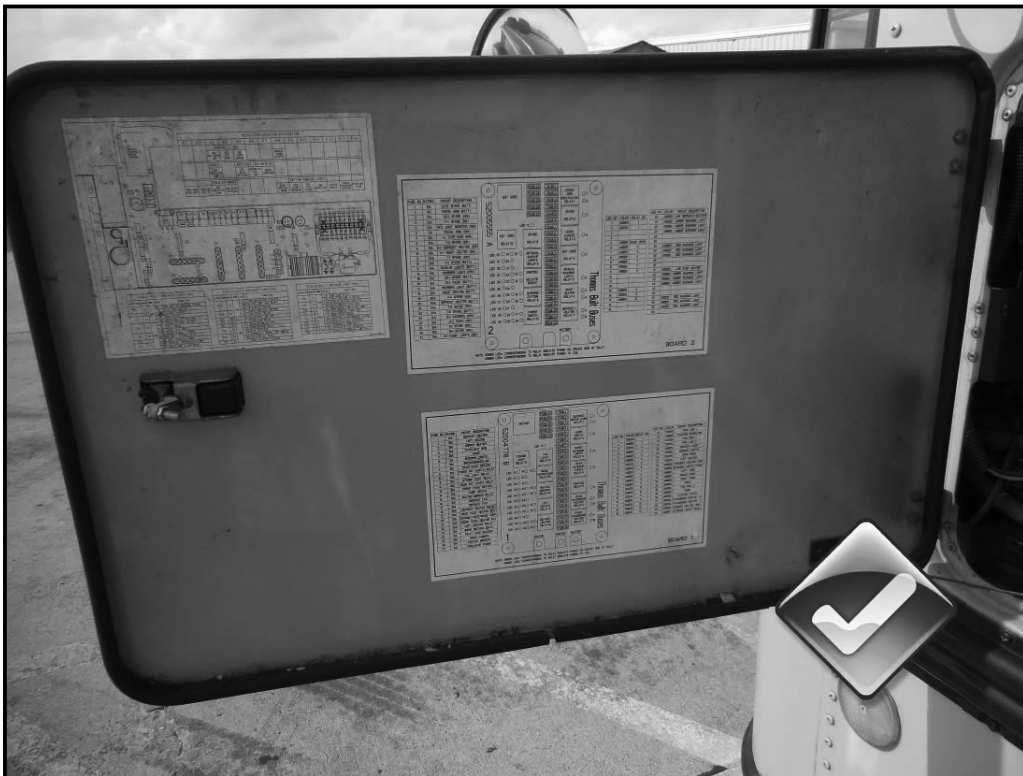
Figure: 12: Acceptable - Example of Fusing labeling on inside of Electrical Panel Door.
