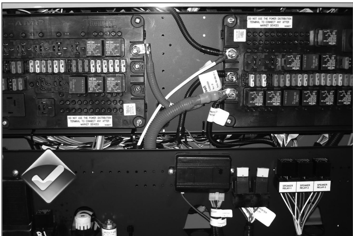
Figure 18: Acceptable - Example of proper OEM electrical connections without Add-on connections.
