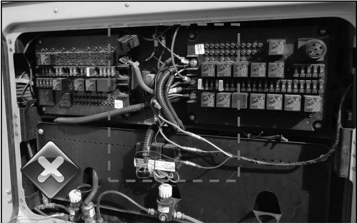
Figure 17: Unacceptable - Add-on connections attached to the power, ignition, and ground studs.
