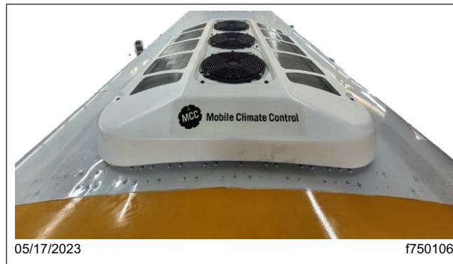
Fig. 4, Vehicle Equipped with Factory-Installed Roof-Top A/C Unit
