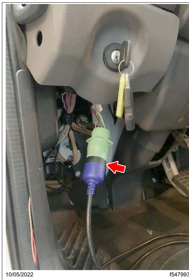
Fig. 1, Connecting the Nexiq USBLink 2 Box to the 9-Pin Connector of the Vehicle
