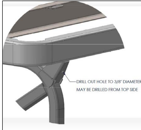
Figure 16: Drilling Location Seat Frame
