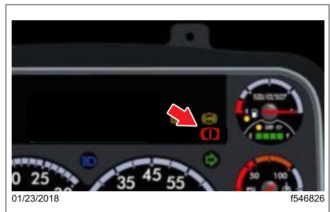
Fig. 2, A Brake Malfunction - OK, No Replacement
