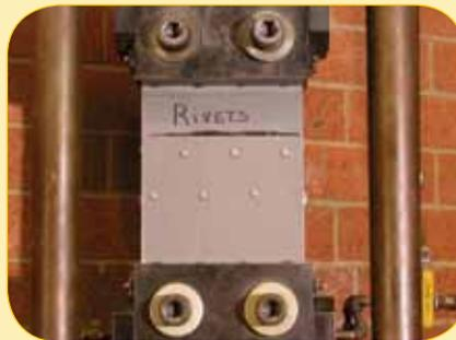
**B RIVETS AFTER:** Rivets after pull test. Rivets at 3.5" overlap, joint tears at an average of 8,462 lbs.
