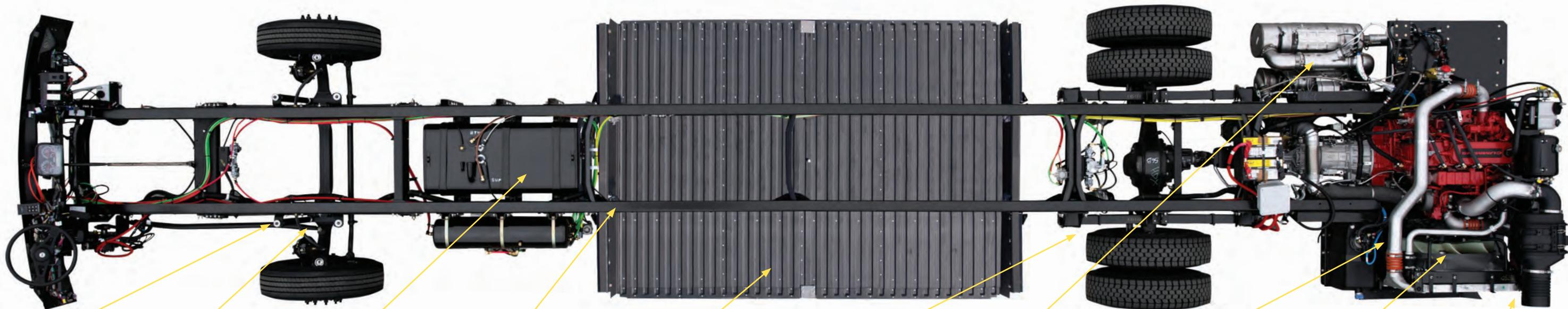
Greaseless front suspension featuring single-stage taper leaf springs (4"x66") with four heavy-duty shock absorbers for outstanding ride quality. Air ride suspensions are available.
