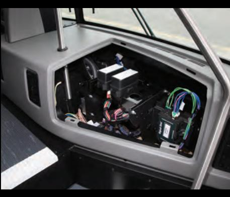
Chassis fuse relay centers and electronic control modules for the intermittent wipers, headlamps and anti-lock brake system are located in a clean, dry environment behind the interior access panel near the stepwell. This easy-to-access location makes maintenance quick and easy.
