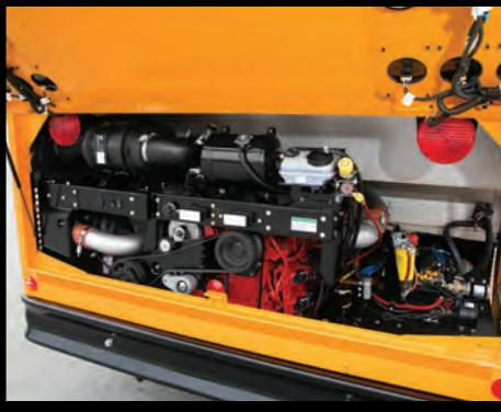
Maintenance shelf allows for quick and easy fluid checks and other routine maintenance. It can also be removed to provide full engine access.
