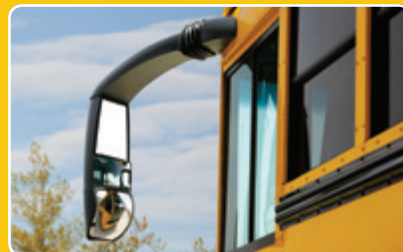
Flat and convex integrated mirrors improve rear-view visibility.
